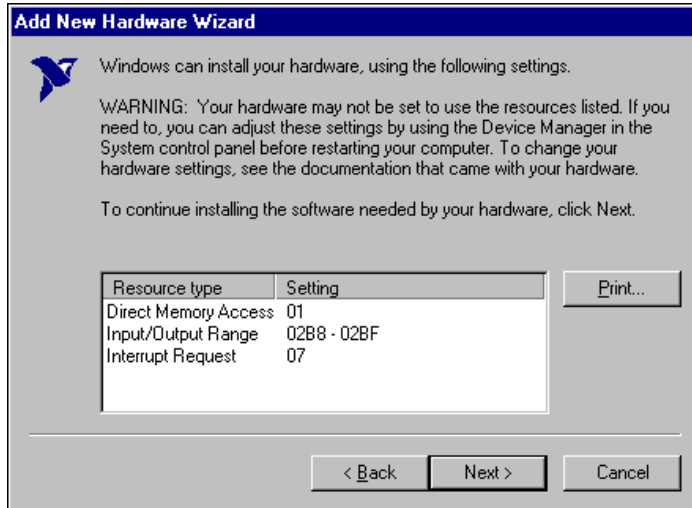
Figure 2-4. PC/104-GPIB Resources Assigned Successfully
